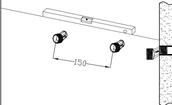
Adjust the position of the two bended connectors to be horizontal, and make sure the center distance to be 150mm.
