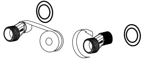
Wrap the bended connector with Teflon tapes. Then twist it into the outlet hole.
