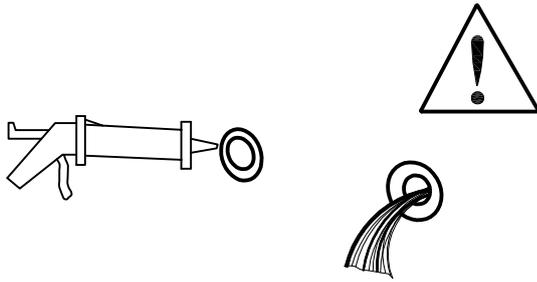
Fill the gap between wall and hole with silicone, Turn on the valve and allow the water to run freely for 5 minutes. Then turn off the valve.
