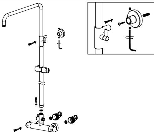
Adjust the straight pipe and connected to the mixer body, then lock the female screw tightly. And connect to the fixing plate. Tighten the grub to the fixing plate. Tighten the grub screw with the allen key.
