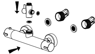
Install the flange to the bended connector, put the flat washer in the inlet hole. Lock the female screw to tight the mixer body.
