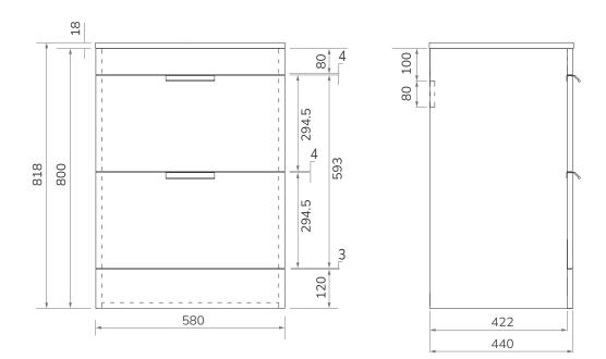
All measurements shown are in millimetres. Drawing sizes are not to scale. Measurement accuracy ±5mm. SONAS Bathrooms reserves the right to make changes and/or modifications to products and specifications without prior notice.
