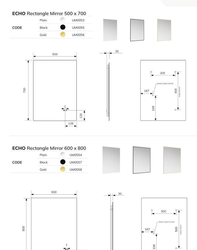
All measurements shown are in millimetres. Drawing sizes are not to scale. Measurement accuracy ±5mm. SONAS Bathrooms reserves the right to make changes and/or modifications to products and specifications without prior notice.
