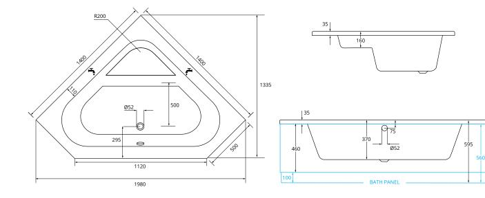
All measurements shown are in millimetres. Drawing sizes are not to scale. Measurement accuracy ±5mm. SONAS Bathrooms reserves the right to make changes and/or modifications to products and specifications without prior notice.
