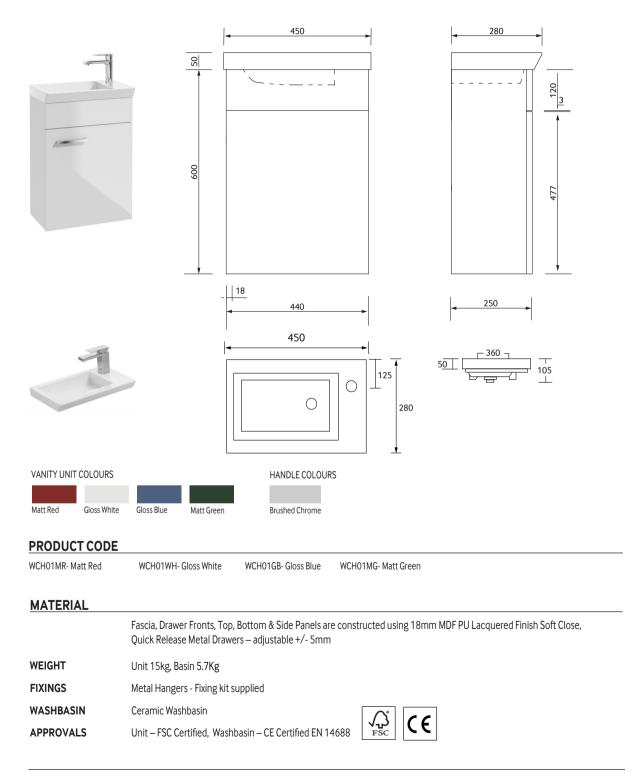
All measurements shown are in millimetres. Drawing sizes are not to scale. Measurement accuracy ±5mm. SONAS Bathrooms reserves the right to make changes and/or modifications to products and specifications without prior notice.
