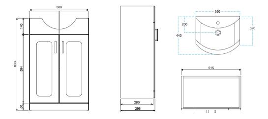
All measurements shown are in millimetres. Drawing sizes are not to scale. Measurement accuracy ±5mm. SONAS Bathrooms reserves the right to make changes and/or modifications to products and specifications without prior notice.
